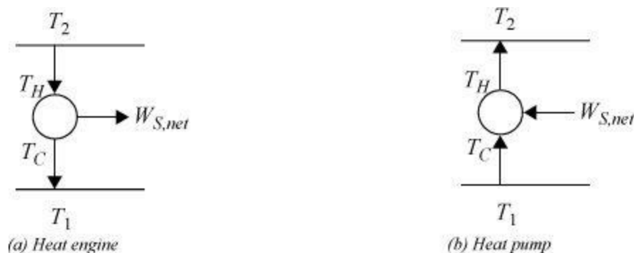
Figure 4.5. Schematic of a heat engine (a) and heat pump (b). The temperatures of the reservoirs are not required to match the reversible engine temperatures, but work is optimized if they do, as discussed in the text.
