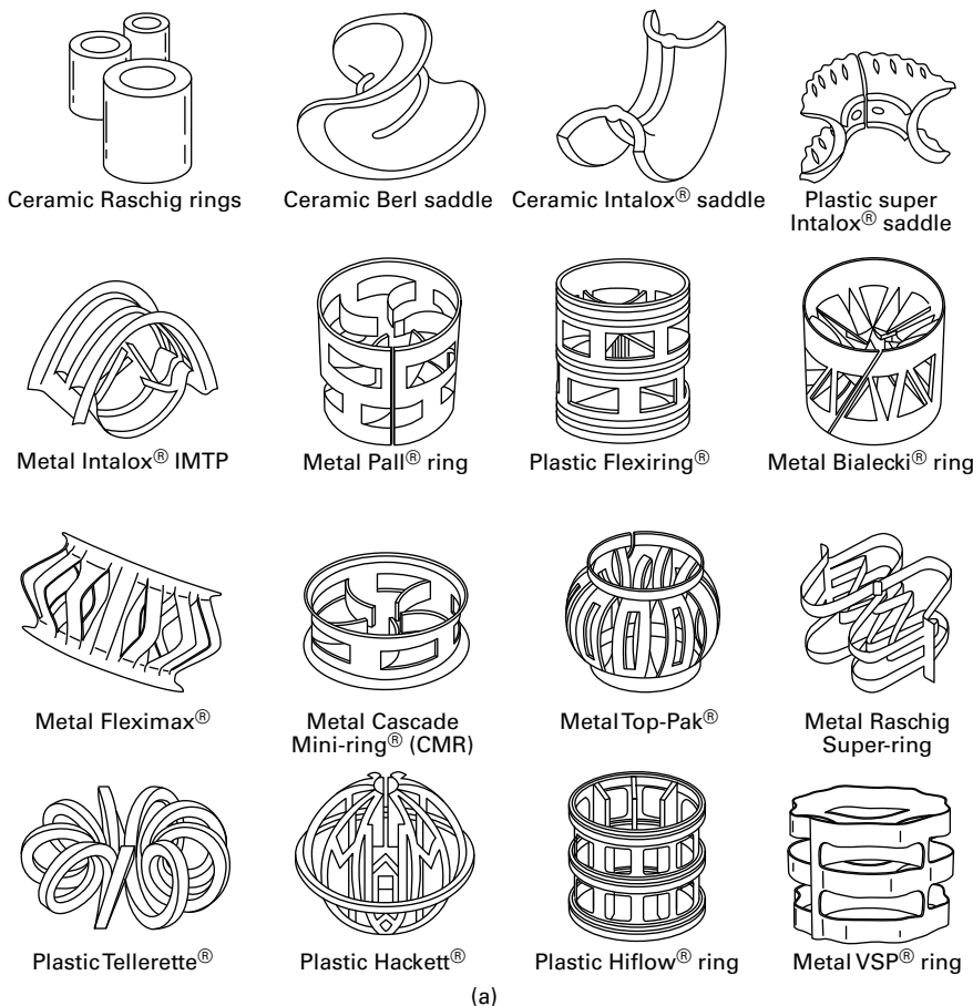
Figure 6.7 Typical materials used in a packed column: (a) random packing materials; (continued)
