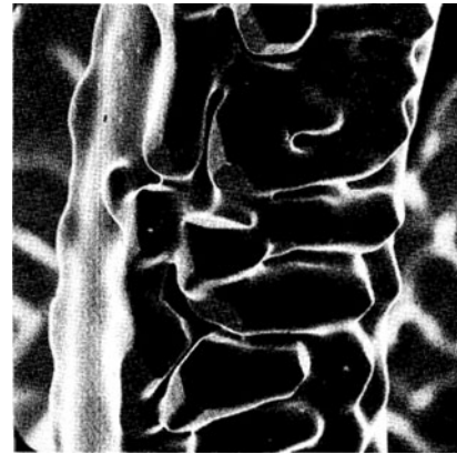
Figure 16.14 V-shaped grooves and holes after 3,500 hours at 3,000 K. Reprinted with permission (Garbe, 1980).
