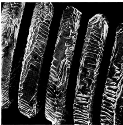
Figure 16.12 Faceted structure after 3,096 hours at 3,000 K. Reprinted with permission (Garbe, 1980).
